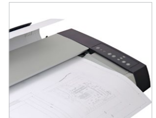
Intelligent paper return does away with paper rewinding
